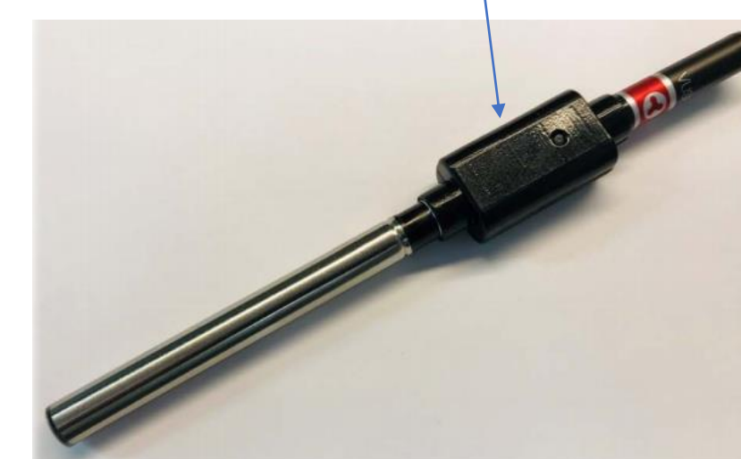
Figure 2. The PUB instrument is shown, inserted between a Vuse Solo cartridge and the power unit.
