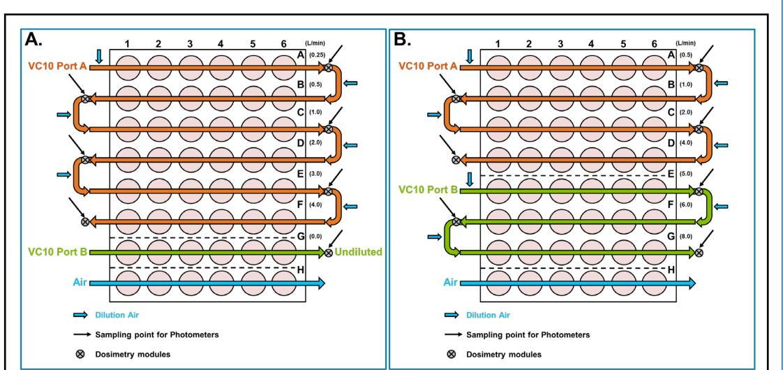
Figure 2: WA exposure module. Mammalian 6/48 WA exposure module set up for HTP (A) and combustible cigarette (B) exposures. HTP WA was serial diluted through rows 1 - 6 (0.25 to 4.0 L/min dilution airflows) or undiluted (0 L/min) in row 7. For combustible cigarettes, WA was serial diluted through rows 1 - 4 (0.5 to 4.0 L/min) and rows 5 - 7 (5.0 to 8.0 L/min). Row 8 (A & B) was used for air controls.
